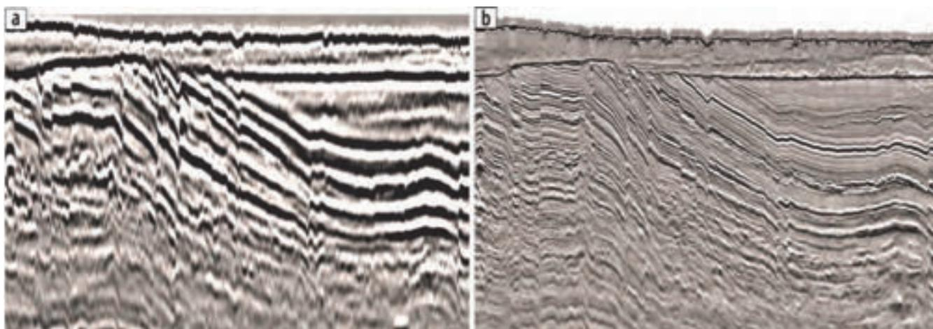
**Figure 2.** (a) Conventionally acquired and processed exploration 3D seismic data. (b) UHR3D data from the same location. Data courtesy of TGS.
