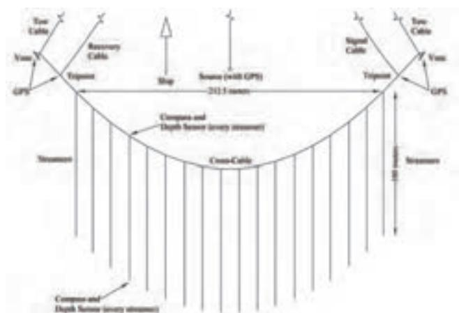
Figure 1. Scaled towing schematic for an 18-streamer UHR3D array. Modified from Brookshire et al., 2015.
