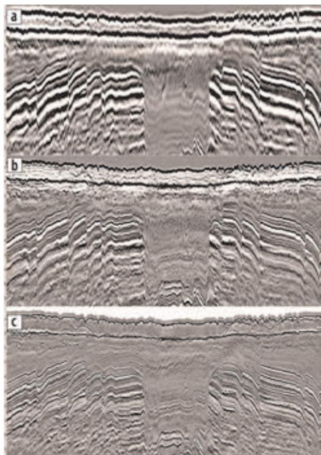
**Figure 3.** (a) Conventionally acquired and processed exploration 3D seismic data. (b) The same conventionally acquired 3D exploration data reprocessed for high-resolution. (c) UHR3D data from the same location. Data courtesy of TGS.
