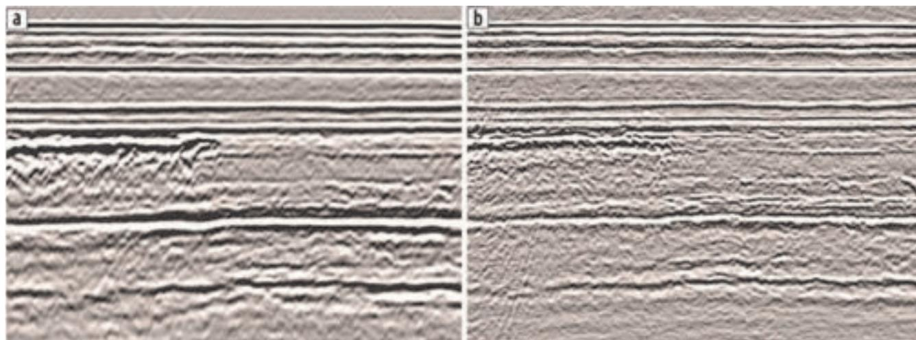
**Figure 4.** (a) High-resolution 2D data traditionally used for geohazard assessment and well clearance. (b) UHR3D data from the same location. Data courtesy of Statoil.
