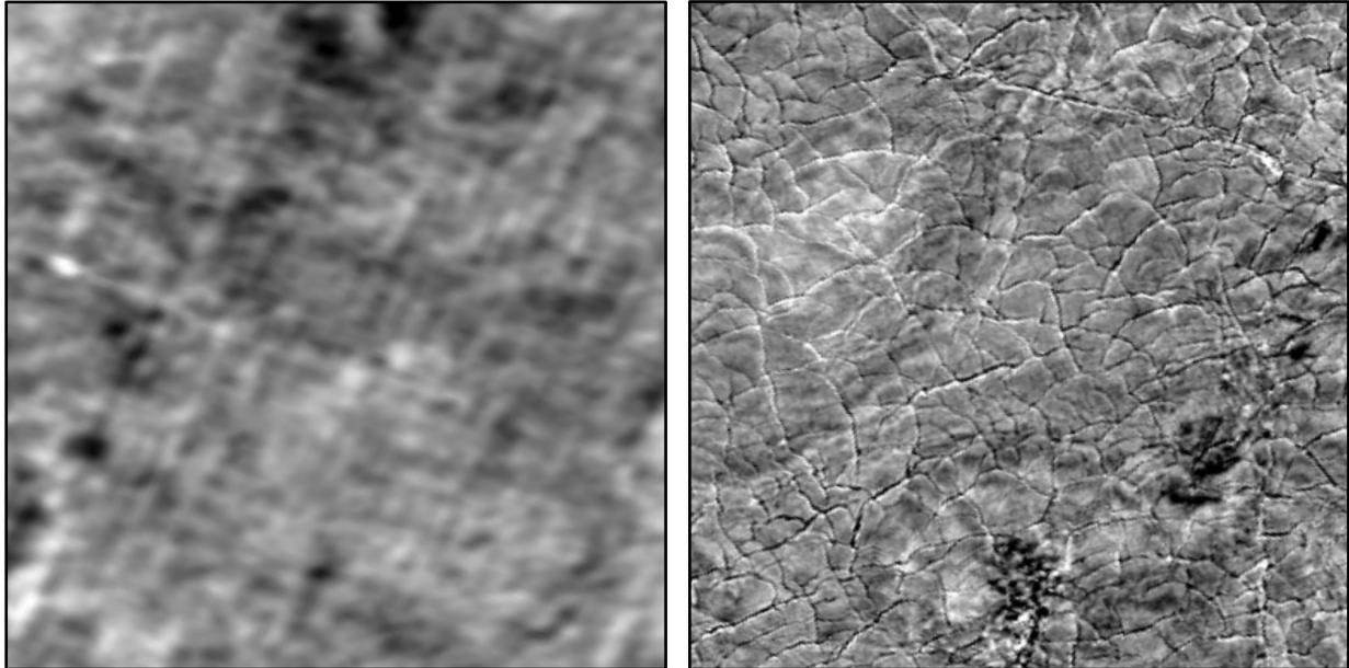
**Figure 2:** Time slice comparison of convention streamer 3D seismic with broadband processing (left) and P-Cable 3D seismic with broadband processing (right). Image courtesy OMV.
