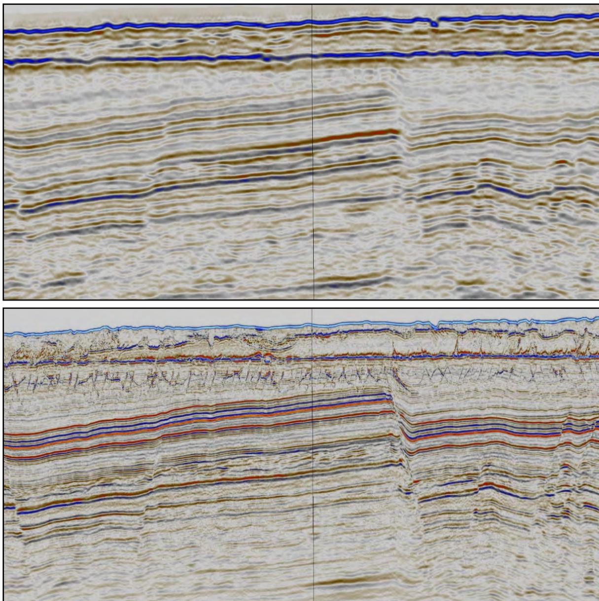
**Figure 1:** Vertical section comparison of convention streamer 3D seismic with broadband processing (top) and P-Cable 3D seismic with broadband processing (bottom). Image courtesy OMV.
