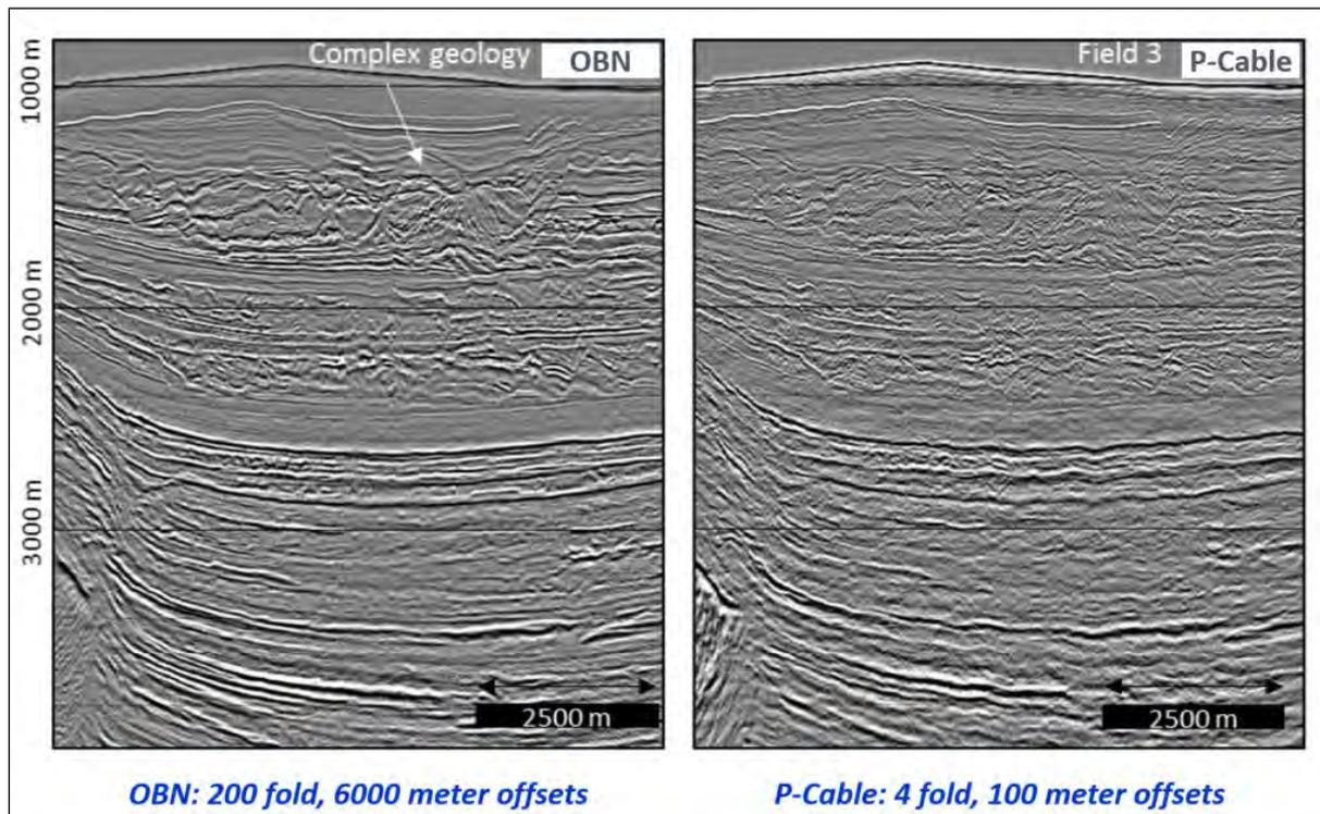
**Figure 3:** Vertical section comparison of full offset, rich azimuth OBN 3D seismic with broadband processing (left) and P-Cable 3D seismic with broadband processing (right). Both datasets were pre-stack depth migrated using the same velocity field. Image courtesy Shell.
